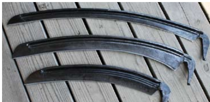
Above: three US made blades. Below: one of 1000 blades imitating the US form, made by Scröckenfux for Compass for sale in the UK, in about 2002, after the stock of patent Tyzack rivetted blades ran out. It is reduced from £30 to £18 and described as a “rivetted” blader, which, of course, it isn’t.
